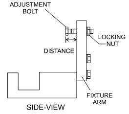
Figure 42. Trowel Arm Adjustment Tool Side View
